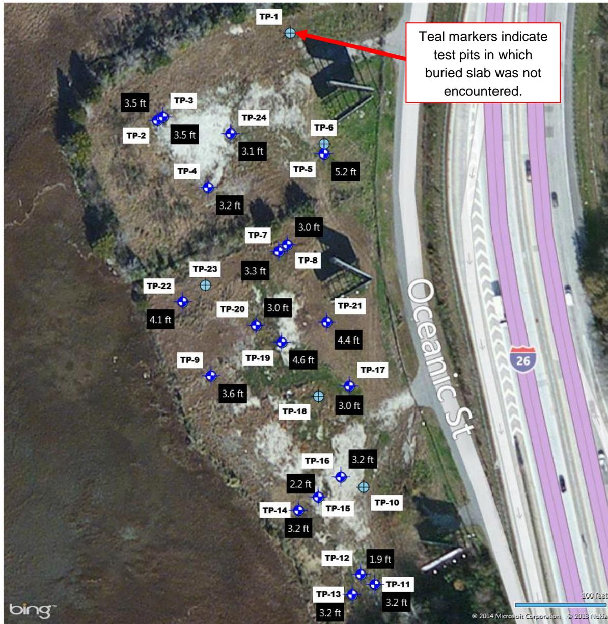
**Figure 1.** Approximate Depths to Encountered Buried Concrete Slab
